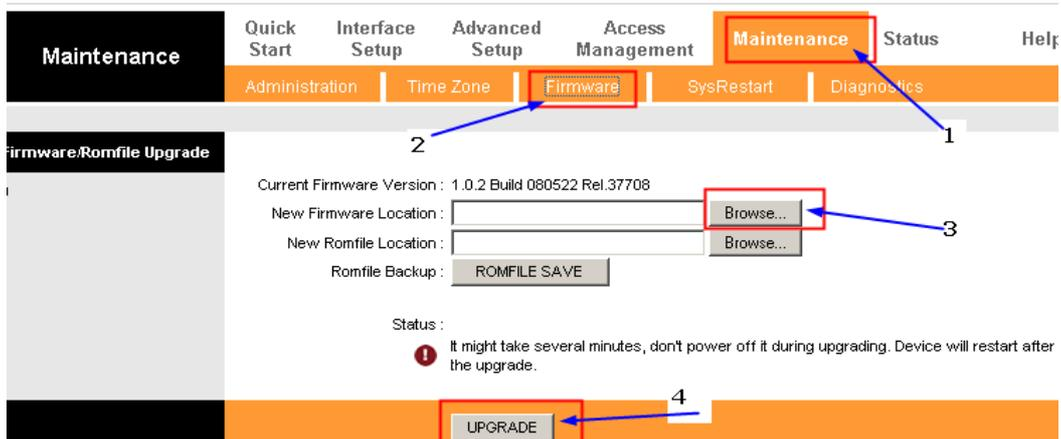
**Step 3** Click the **UPGRADE** button. The device will reboot automatically after the upgrading has been finished. Please wait about 3 minutes.
